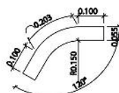
Code: Arc 120°-5575 / Puzzle light 11 w/m, 1350 lm/m
